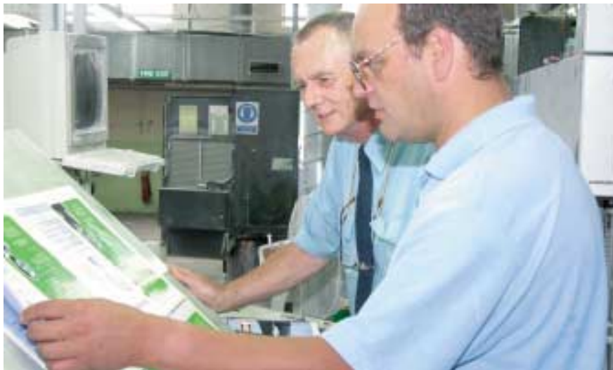
Derek Smail and Graham Sutton (Machine Minder) checking the colour densities of a job running on press
